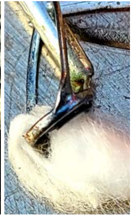
A cotton swab can be used to find a cracked line guide.
